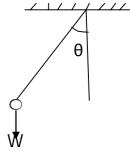
**<u>Ans:-</u>** A simple of pendulum of length I is suspended from a rigid support.
